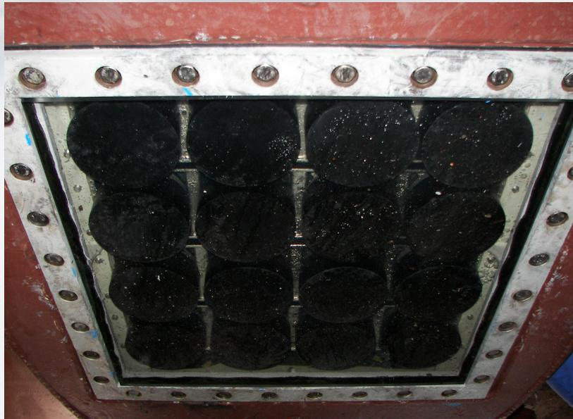
The EdgeTech 3300 hull mount sub-bottom profiling system is a versatile wideband Frequency Modulated (FM) sonar that generates cross-sectional images of the seabed and collects digital normal incidence reflection data over many frequency ranges. EdgeTech's Full Spectrum® Technology has several distinct advantages over conventional sub-bottom systems, including increased penetration and higher resolution.
