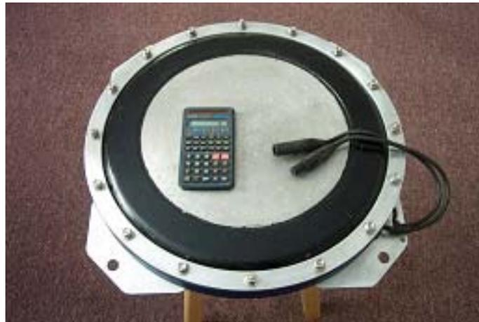
**Figure 2 The IKB Model B3 Boomer Source**
